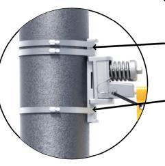
At minimum, you should install 2 straps on "outer" or spring side of the unit. This is where the most tension is on the unit. You can have 1 or 2 straps on the "inner" side.
