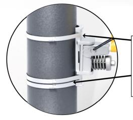
At minimum, you should install 2 straps on "outer" or spring side of the unit. This is where the most tension is on the unit. You can have 1 or 2 straps on the "inner" side.
